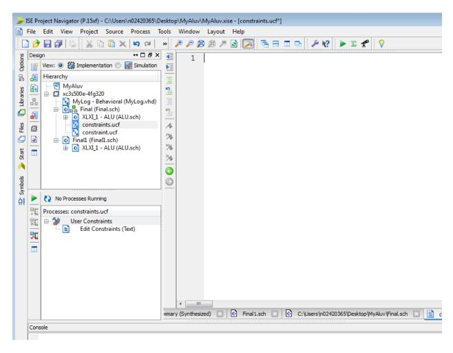
Here you can assign inputs and outputs to appropriate switches and LEDs in the FPGA chip.
