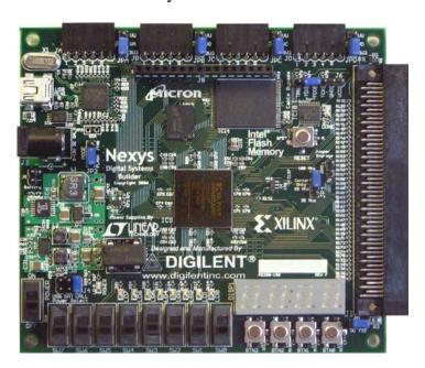
1. Now that through simulation you have verified that your design is working, the next step is to download your design into the FPGA (Field Programmable Gate Array) of the NEXYS 2 Board. Save your schematic and return to the Project Navigator. Change your view back to implementation. Before proceeding, once again make sure that the FPGA device under sources is listed as XC3S50e-4fg320. If not double click on the device and make corrections as follows
