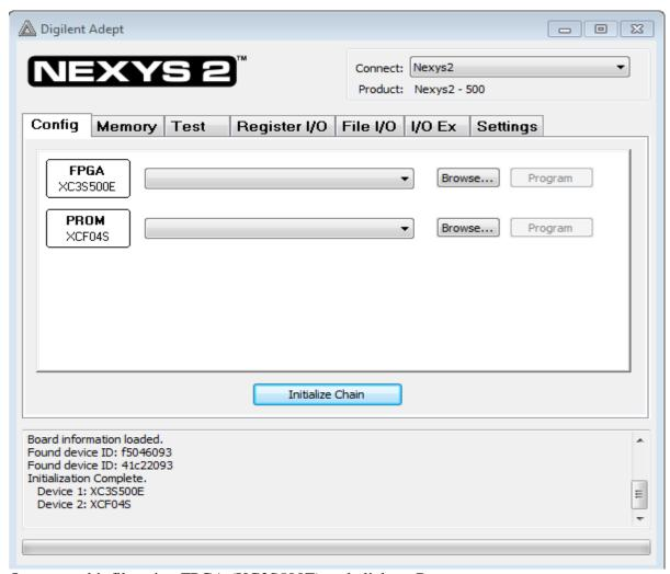
Open your bit file using FPGA (XC3S500E) and click on Program.
